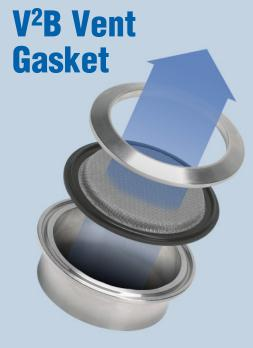
The Rubber Fab V2B Vent Gasket provides vacuum and pressure relief for **pharmaceutical** and **food/beverage processing** tank venting when **airborne particulate removal is required**. A 200 mesh screen combined with a 14 mesh screen of **sintered construction** creates a cost effective alternative to expensive vacuum breakers and venting systems.
